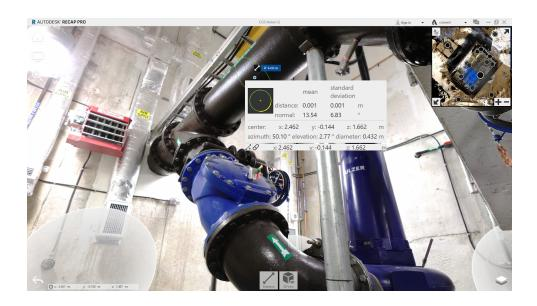
Other measurement tools include *3-Point* and *Faces*. The *3-Point* tool can be used to determine the angle between three points and the *Faces* tool measures the angle between two surfaces.
